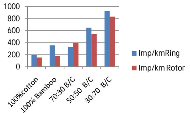
Graph 3. Unevenness (U%) of Ne 16 for Ring and Rotor spun yarns
