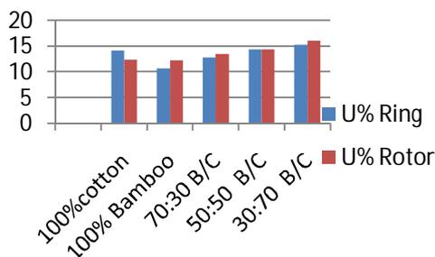
Graph 1. Yarn unevenness(U%) and for Ne 10 ring and rotor spun yarns.
